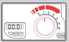
When you turn the Control Dial (16) to start mixing, the Timer (15) will automatically start counting up.
