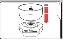
Place the Motor Housing onto a dry stable, surface. Ensure the Drive Shaft is fitted in the Mixing Bowl and lower the Mixing Bowl onto the Motor Housing, ensuring the Mixing Bowl is properly seated (see 'Mixing Bowl Setup' section on page 7).
