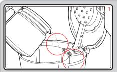
Fill the Water Reservoir (5) with cold water. Do not overfill.
