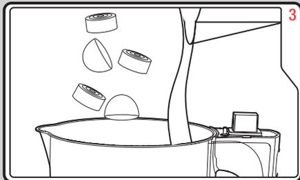
Place all the ingredients into the Jug (15). Add the liquid last, filling up to between the Min and Max marks on the Jug (15).
