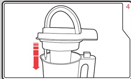
Place the Lid (9) back onto the Jug (15) ensuring it is securely in place.
