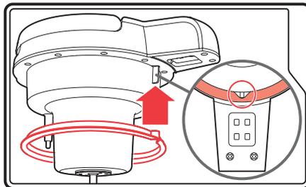
Also ensure that the flat ridge part of the Lid Seal (12) is at the lowermost position.
