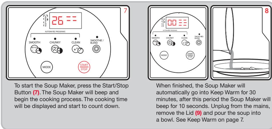
To start the Soup Maker, press the Start/Stop Button (7). The Soup Maker will beep and begin the cooking process. The cooking time will be displayed and start to count down.
