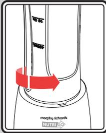
Turn the Beaker (2) anti-clockwise to release & lift away from the Main Unit (5).
