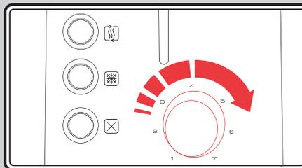
Adjust the Browning Control (3) to the desired setting.
